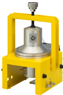
AFS 153 media tester and typical MPPS curves.
