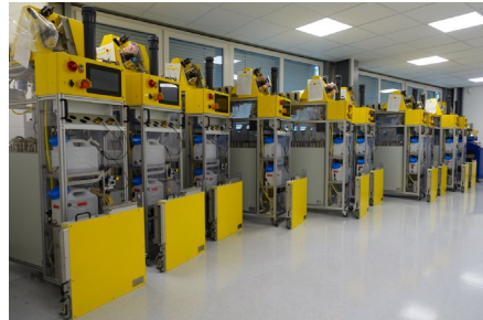
Measuring stations for fully integrated quality control of medical filters
